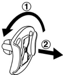
① Rotate the packaging lock anticlockwise 90 degrees
